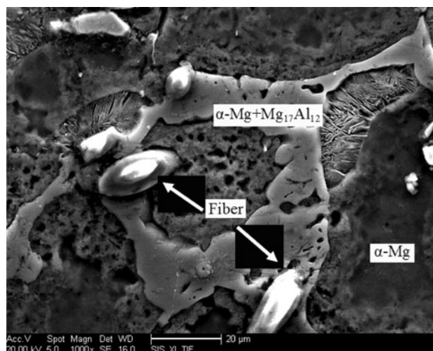
Fig. 2 Microstructure of squeeze casting formed Al 2 O 3sf /AZ91D with 10% Al 2 O 3sf with an applied pressure of 60 MPa
