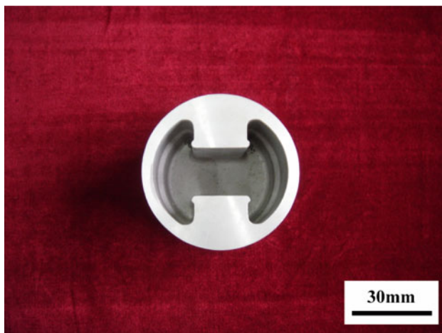
Fig. 7 Automotive piston component made from \text{Al}_2\text{O}_{3\text{sf}}/\text{AZ91D} and thixoforged under an applied pressure of 350 MPa
